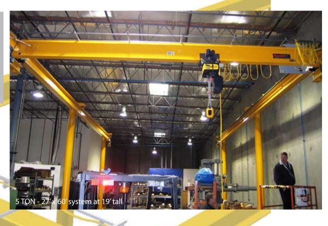
T-TRAC SERIES bridges ship complete from the factory including all festooning and control components therefore requiring less labor during installation. Ergonomic slim line pendants including all 2-speed buttons with On/OFF come standard on the T-TRAC.. The 1HP AC motors compliment the drive train of the T-TRAC and are controlled by state of the art variable frequency drives.
