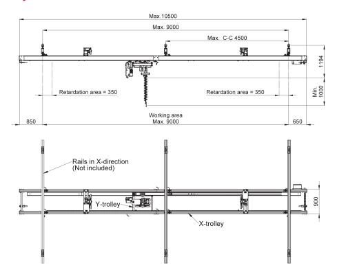
This lifting device is delivered pre assembled, and includes one lifting motor and three motors for the X and Y movements.
