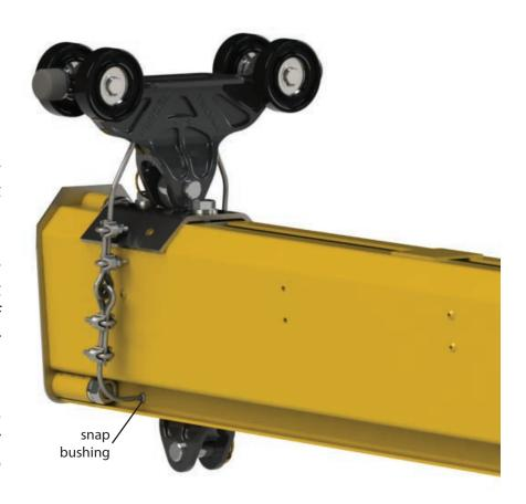
**Note to installer:** Make sure that all threaded connections internal or external have been treated with a locking agent such as Loctite<sup>®</sup>. Small 3/8" holes will need to be drilled thru the rail in order to allow the safety cable to pass thru and then re-attach back onto itself. The cable provided will pass thru the trolley/endtruck body through the designated arc shaped channel immediately above the hook. Please use the snap bushings for each hole drilled.
